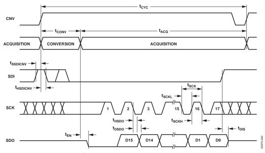
Figure 25. CS Mode 4-Wire with BUSY Indicator Serial Interface Timing
