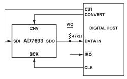
Figure 24. CS Mode 4-Wire with BUSY Indicator Connection Diagram
