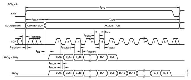
Figure 27. Chain Mode, No BUSY Indicator Serial Interface Timing
