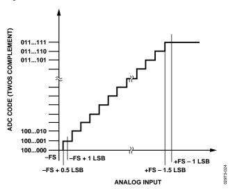
Figure 13. ADC Ideal Transfer Function Figure 14. ADC Ideal Transfer Function
