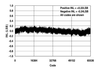
Figure 7. Integral Nonlinearity vs. Code
