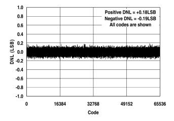
Figure 10. Differential Nonlinearity vs. Code
