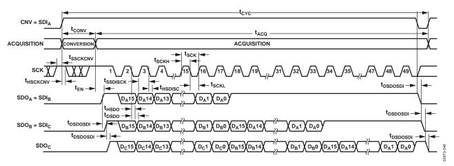
Figure 29. Chain Mode with BUSY Indicator Serial Interface Timing
