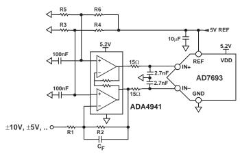
Figure 17. Single-Ended-to-Differential Driver Circuit
