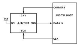
Figure 18. CS Mode 3-Wire, No BUSY Indicator Connection Diagram (SDI High)
