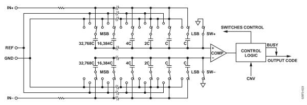
Figure 12. ADC Simplified Schematic
