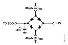
Figure 3. Load Circuit for Digital Interface Timing
