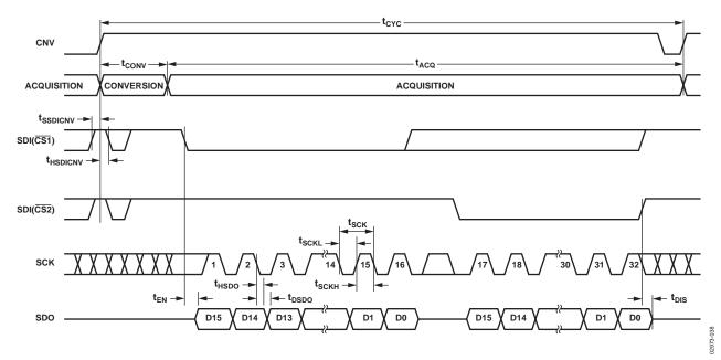
Figure 23. CS Mode 4-Wire, No BUSY Indicator Serial Interface Timing
