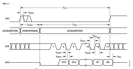
Figure 21. CS Mode 3-Wire with BUSY Indicator Serial Interface Timing (SDI High)
