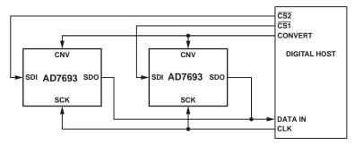
Figure 22. CS Mode 4-Wire, No BUSY Indicator Connection Diagram
