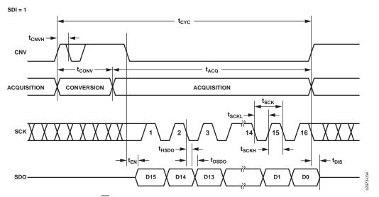
Figure 19. CS Mode 3-Wire, No BUSY Indicator Serial Interface Timing (SDI High)
