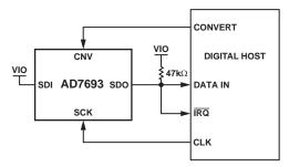
Figure 20. CS Mode 3-Wire with BUSY Indicator Connection Diagram (SDI High)
