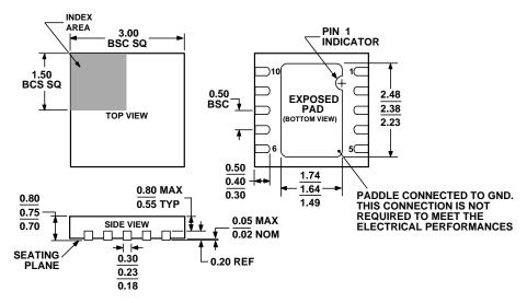
Figure 33. 10-Lead Lead Frame Chip Scale Package [QFN (LFCSP\_WD)] 3 mm × 3 mm Body, Very Very Thin, Dual Lead (CP-10-9) Dimensions shown in millimeters
