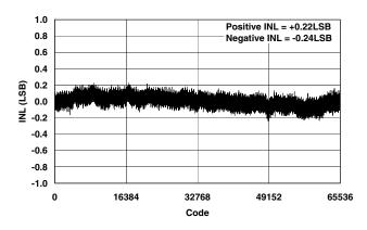
Figure 1.Integral Nonlinearity vs. Code
